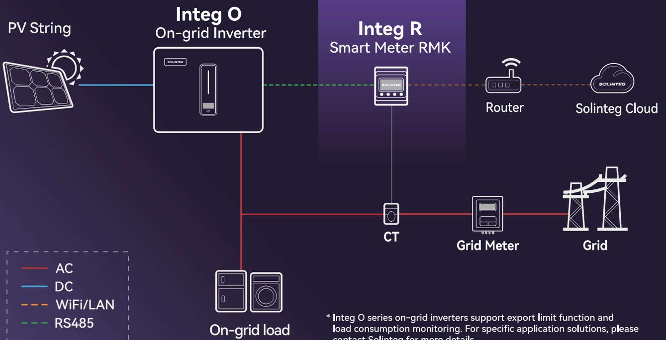
Solinteg smart meter with two versions of RMM and RMK, is used in the whole energy system management and monitor, providing the real-time information.
